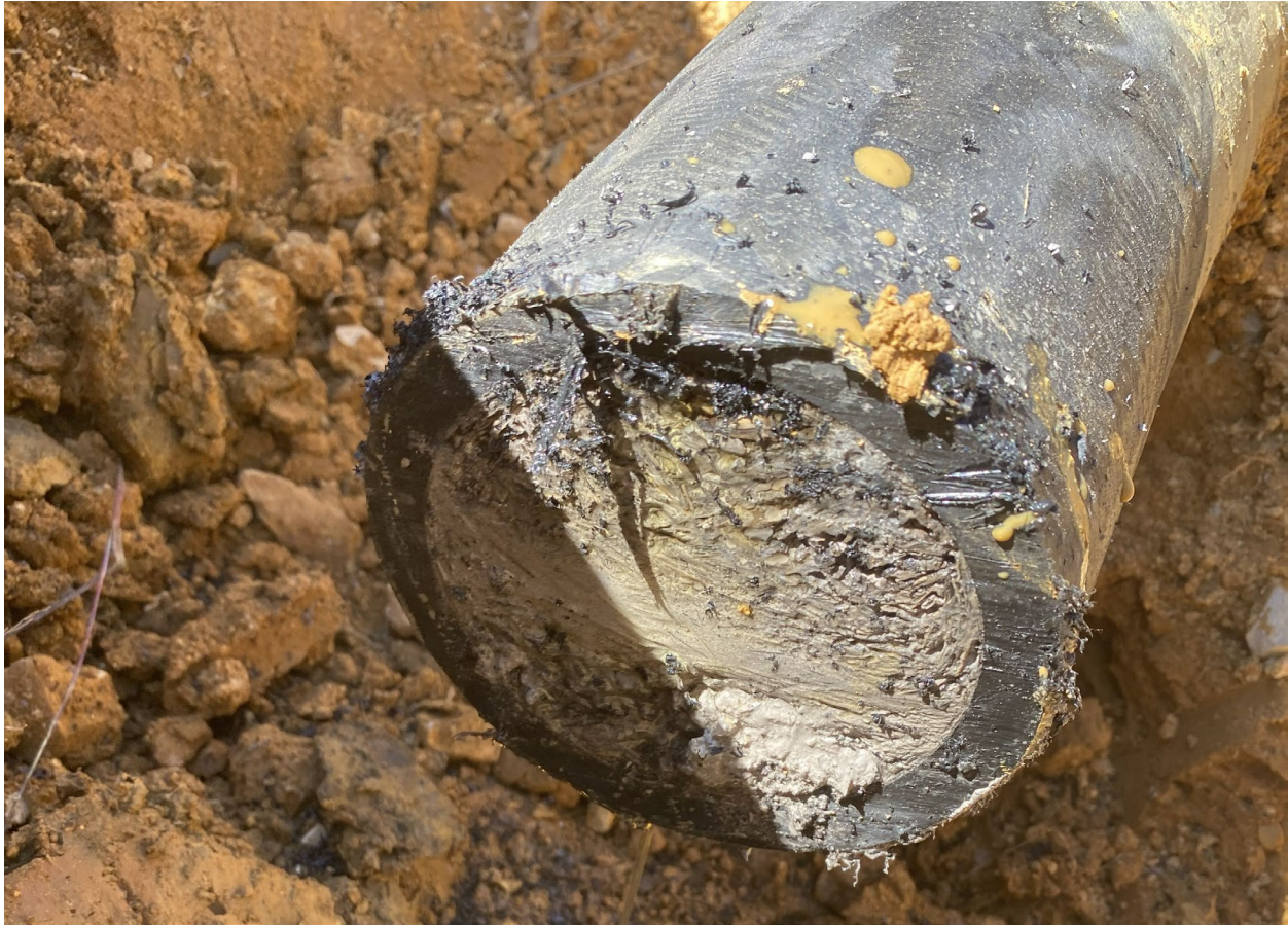
Figure 12. Clogged Forcemain Identified During Construction
