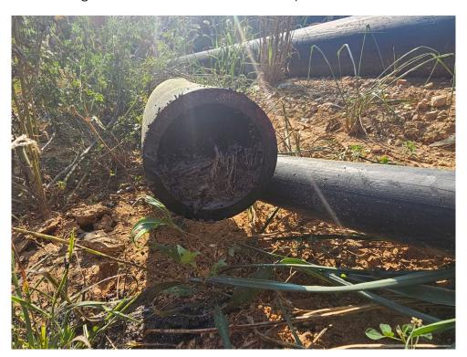
Figure 13. Solids in Landfill Gas Liquids Forcemain
