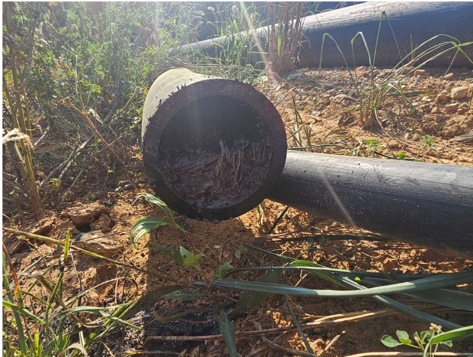
Figure 16. Solids in Landfill Gas Liquids Forcemain
