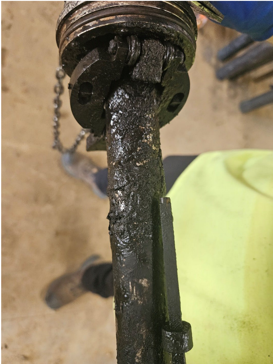
Figure 18. Solids on a Landfill Gas Liquids Extraction Pump
