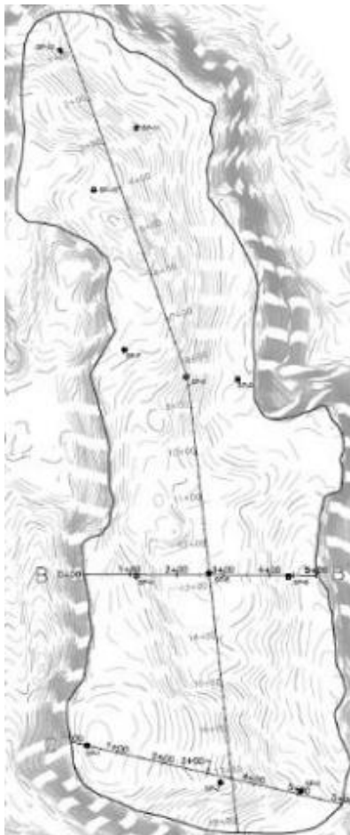
Figure 19. Settlement Plate Locations
