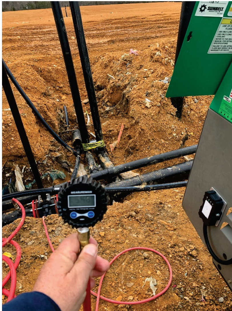
Figure 1. Landfill Gas Pressure Testing - SWP No. 498 Landfill
