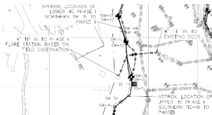
Figure 2. SOMS Phase I As-Built 1
