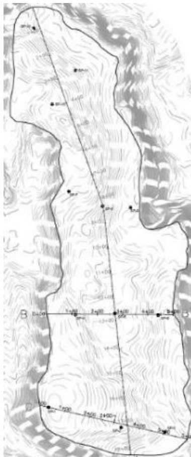
Figure 19. Settlement Plate Locations
