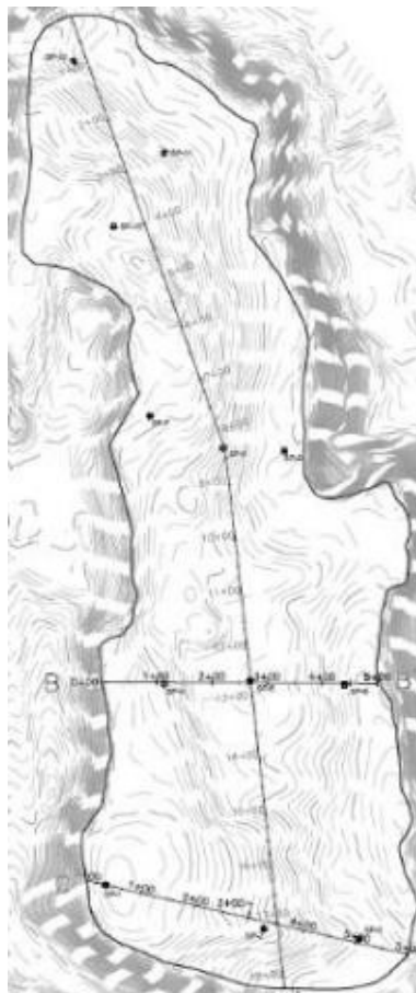
Figure 28. Settlement Plate Locations
