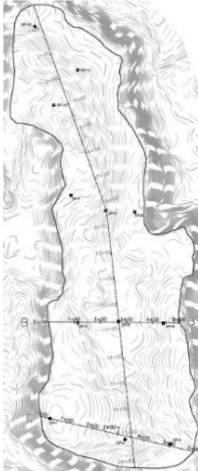
Figure 25. Settlement Plate Locations
