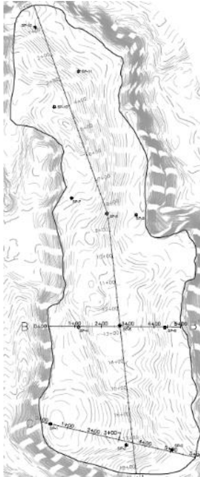
Figure 21. Settlement Plate Locations
