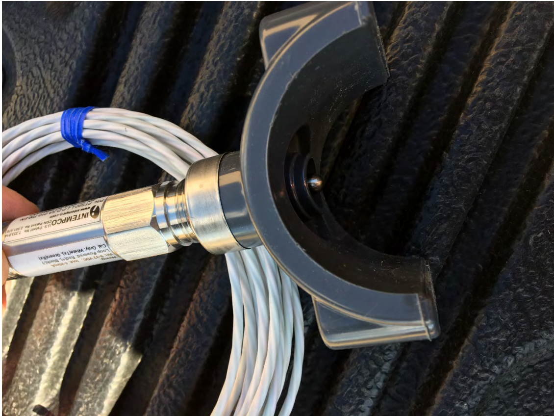
Figure 3. Wellhead Temperature Sensor and Adaptor Saddle
