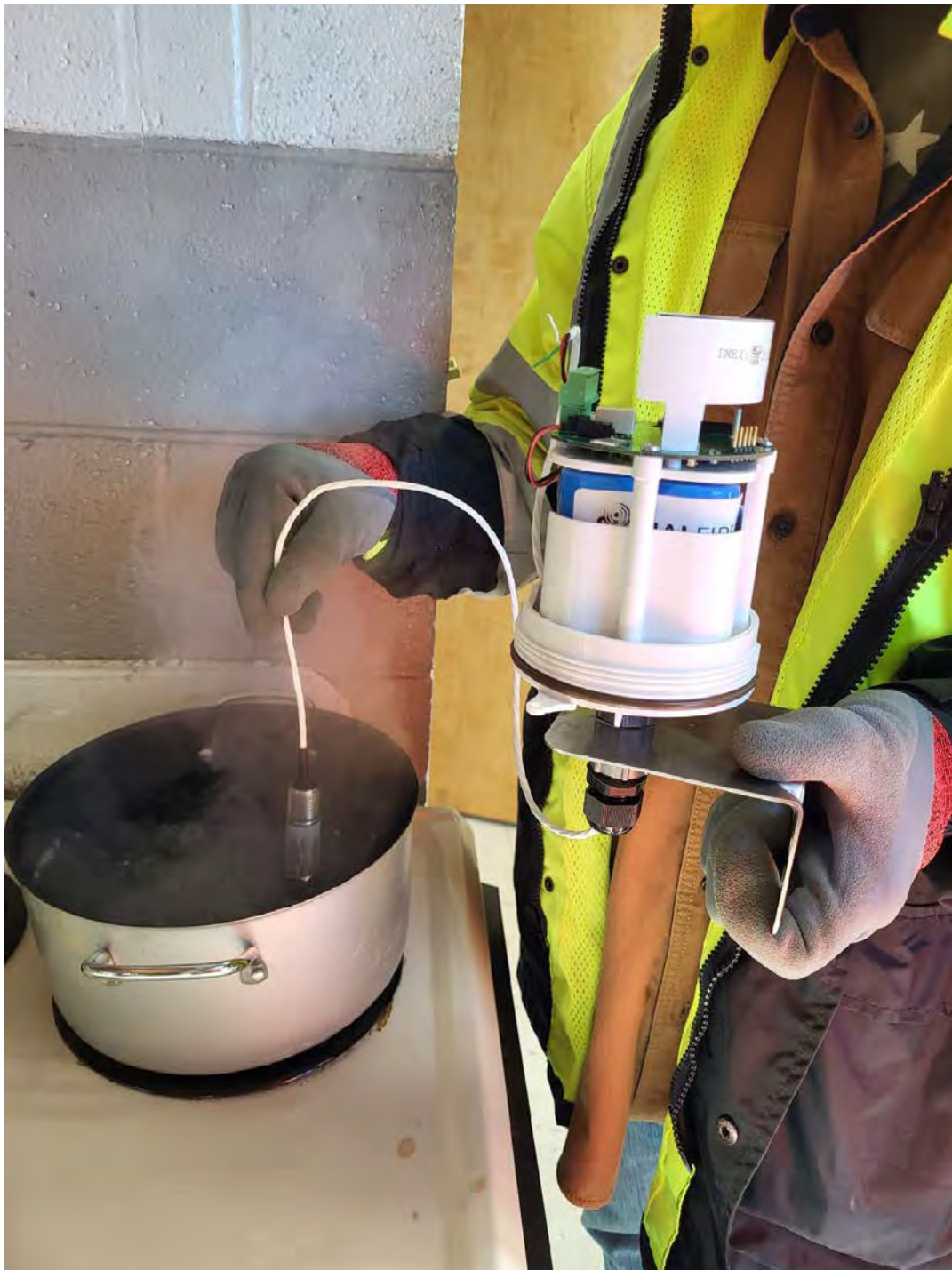
Figure 6. Testing Accuracy of Temperature Sensor using Boiling Water
