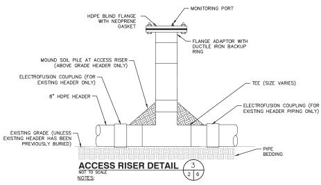
1. CONTRACTOR SHALL INSTALL 10 ACCESS RISERS ON 8 HEADER PIPE AT INTERSECTIONS AND OTHER CRITICAL JUNCTIONS, AS DIRECTED BY ENGINEER. APPROXIMATELY 7 OF THESE WILL BE AFFILIATED WITH NEW HEADER BEING INSTALLED BY CONTRACTOR AND THE REMAINING 3 WILL BE AFFILIATED WITH EXISTING HEADER PIPING
