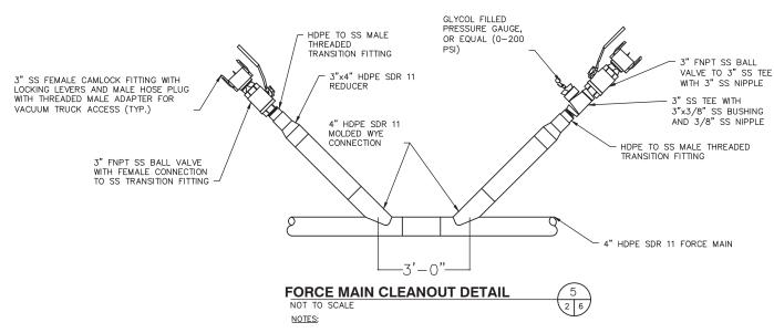
IF CLEANOUT IS INSTALLED GREATER THAN 2 FEET ABOVE GRADE, INSTALL 4"x4" TREATED TIMBER POSTS AND SECURE PIPING AND FITTINGS TO POSTS WITH WORM GEAR CLAMPS.
