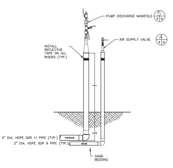
STUB-UP FOR ABOVE GRADE AIR AND FORCEMAIN PIPING DETAIL
