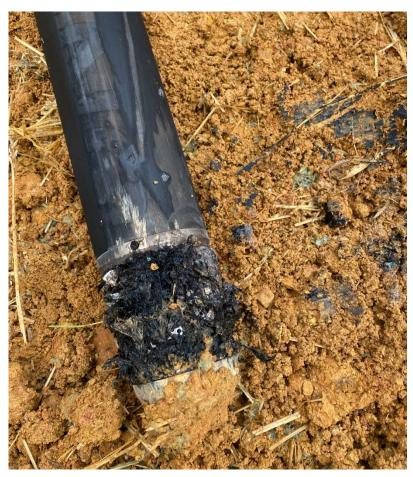
Figure 2. Material Clogging Landfill Gas Well Dewatering Pump
